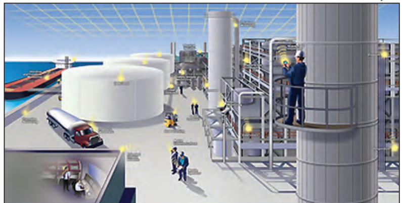
FIGURE 2. This illustration of the "Intelligent Plant" showed the interconnectedness of gas monitoring with other systems such as video surveillance; flow, temperature and vibration monitors; transportation; fire and smoke; and other security systems, calling for a one system approach
