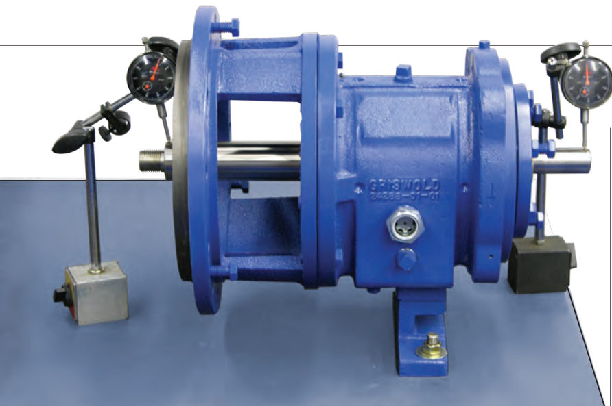
FIGURE 4. Shaft run-out must be checked at both the coupling end and the mechanical seal end. Maximum run-out is 0.002 in. total indicator reading (TIR)
