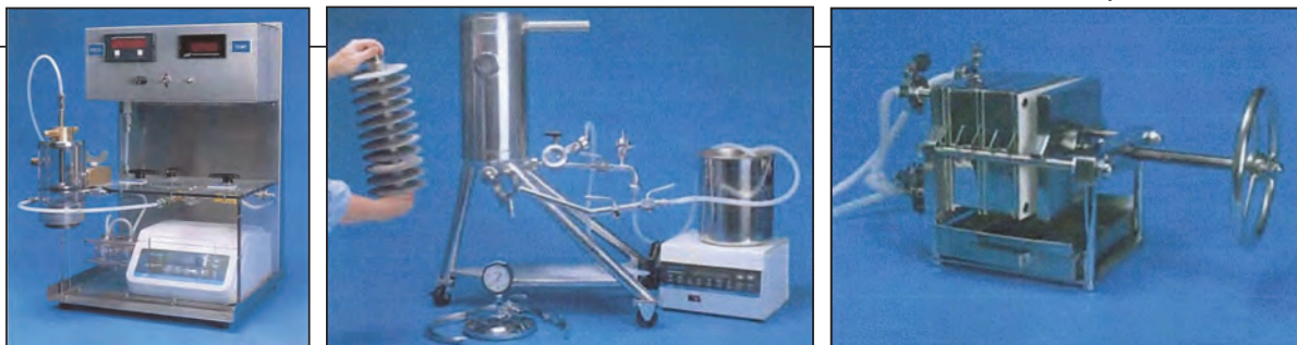
FIGURE 1. Laboratory testing is crucial for the design of a filtration system. Shown here are a Walton test filter station (left), a horizontal-leaf pressure filter test stand with multiple plates (middle), and a plate-and-frame test stand with two plates (right)
